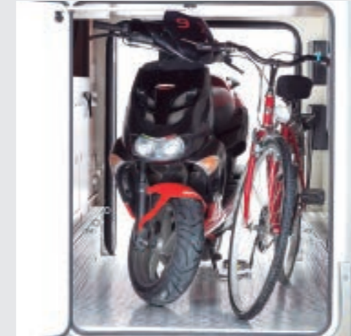
1 Locker with load platform flush with no step. Garage with lighting.
