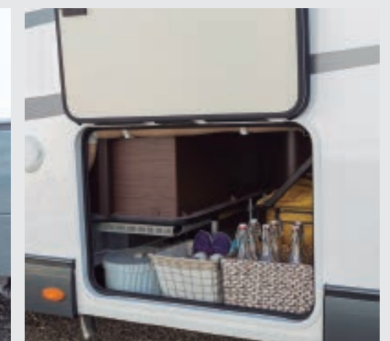
8 AL-KO frame with double pass-through floor K. Yacht Tekno Design.
